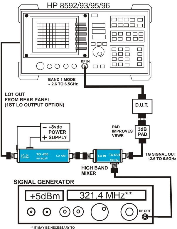
\*\* IT MAY BE NECESSARY TO TUNE IN THE FREQUENCY. TUNE FOR MAXIMUM AMPLITUDE WITH THRUOGH AS DUT
